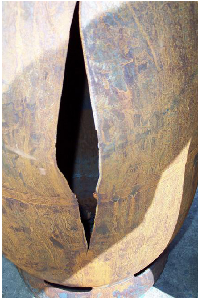
Fig. 9. The appearance of the tear on the burst tank.
